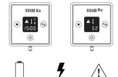
FIGURE 3 - LOW BATTERY & CHARGING INDICATORS
